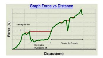
Real time graph (Prostate phantom device test bed) - of force as function of needle depth penetration.
