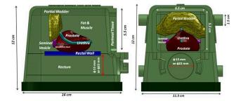
Internal tissues setup of the Brachytherapy prostate phantom. Diameter of 15 mm or 22 mm according to client demand.
