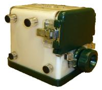
Yezitronix' Model S-MM-2.3-with-Catheter Ultrasound Prostate Phantom is a multiple usage phantom developed for simulation and training.
