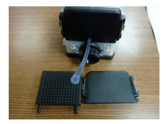
The Catheter Tubing coming out of the removable front window through a matching hole
